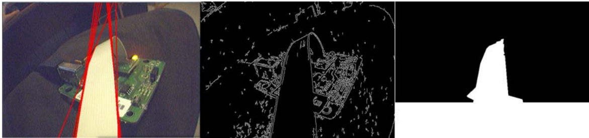
Figure 5 Left: Hough Transform image, Center: Intermediate image, Right: Final image
