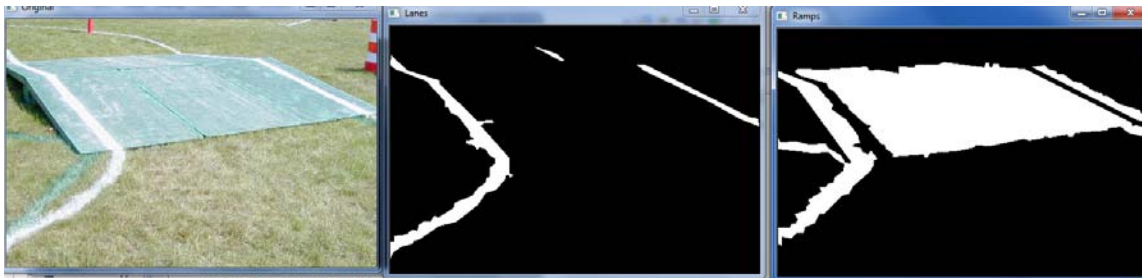
Figure 6 Left: Original image, Center: Final lane detection, Right: Final ramp detection
